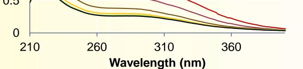
**Change in UV spectrum during the** photochemical iron reduction with respect to time
