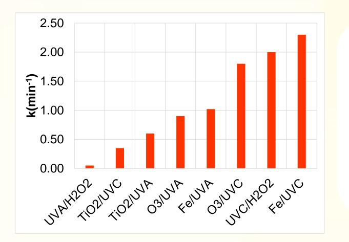
**Comparison of kinetic coefficients** for various AOPs with Fe/UVC
