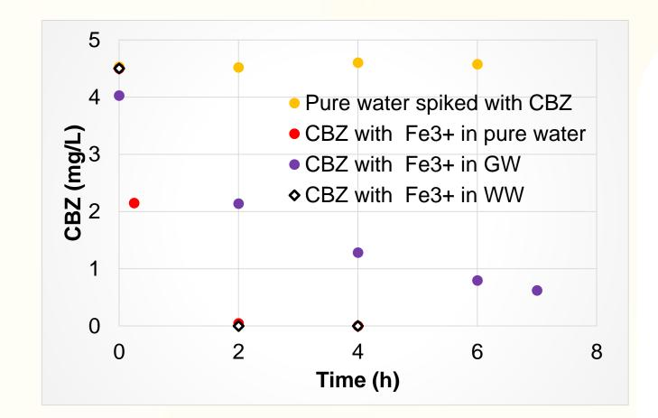
**Degradation of CBZ in various** aqueous matrices by Fe/UVC under sunlight irradiation
