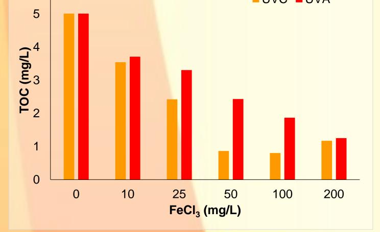
**Reduction in Total Organic Carbon** (TOC) for UVA and UVC irradiations for various ferric ion doses
