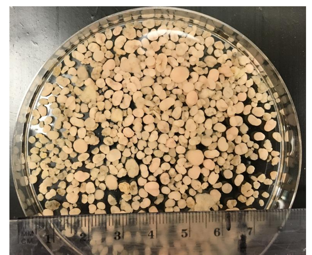
Mature aerobic granules (after 3 weeks of cultivation)
