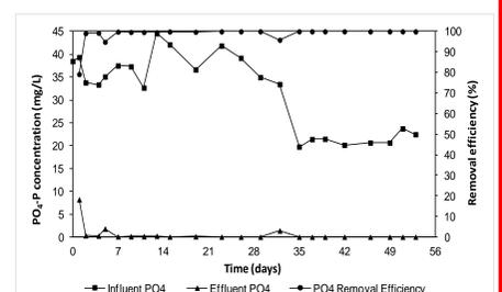
Figure 7 – PO<sub>4</sub>-P removal profile
