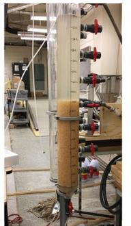
Figure 3 – Aerobic granular reactor: working volume 20 L
