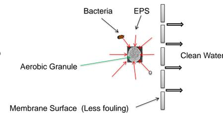
Figure 2 – Mechanism for fouling abatement in AGMBR
