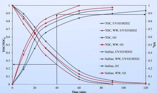
Fig. 5. TOC reduction and sulfate production in the UVC/O<sub>3</sub>/H<sub>2</sub>O<sub>2</sub> process (WW: wastewater samples, [H<sub>2</sub>O<sub>2</sub>] = 2.94 mM, O<sub>3</sub> = 3.7 g/h)
