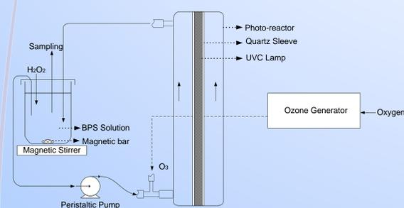
Fig. 4. Schematic of experimental setup
