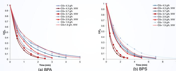
Fig. 3. Effect of O<sub>3</sub> flow rate on the O<sub>3</sub> process in water and wastewater (WW)
