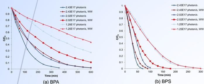
Fig. 1. Effect of light intensity on the UVC only process in water and wastewater (WW)
