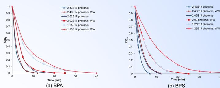
Fig. 2. Effect of light intensity on the UVC/H<sub>2</sub>O<sub>2</sub> process in water and wastewater, [H<sub>2</sub>O<sub>2</sub>] = 0.042 M
