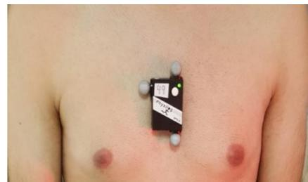
Figure 1: IMU placement on the chest. Three reflective markers are attached to the IMU only for validation of the detected postural transitions using motion capture cameras.
